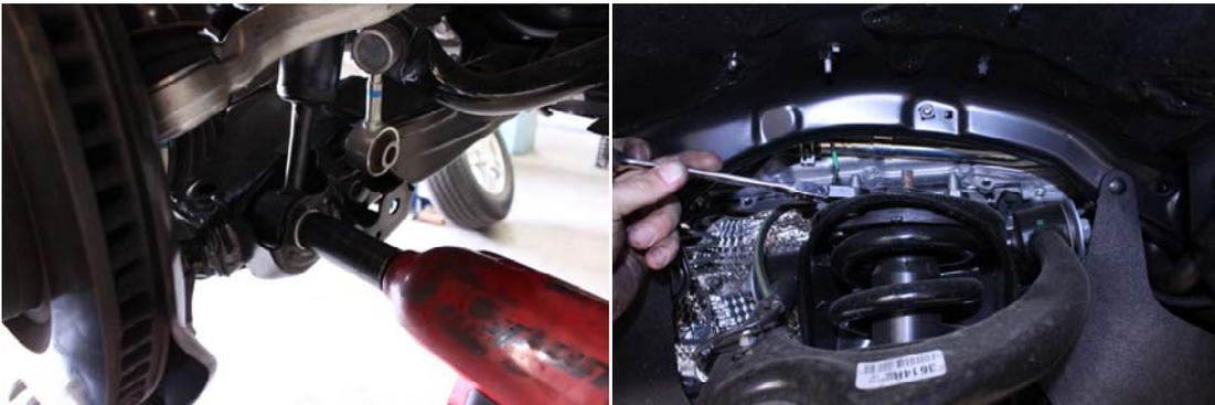
7. Loosen and remove the two 22mm bolts that connect the upper ball joint to the spindle. Holding the strut with one hand, remove the four 14mm upper strut mounting nuts. Remove the strut, being careful not to damage the CV boot on 4WD models.
