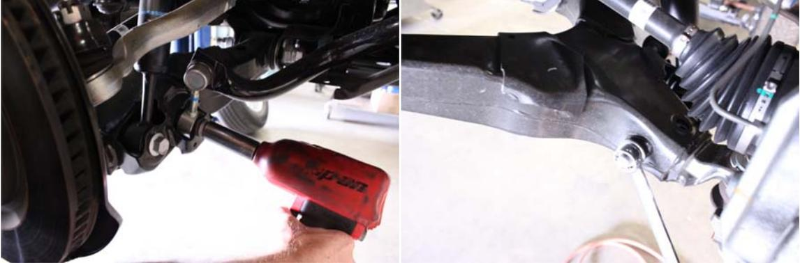
3. Using a 24mm socket, loosen but don't remove, the driver side lower control arm bolts. This will allow the lower control arm to move freely, **do not remove alignment cams.**
