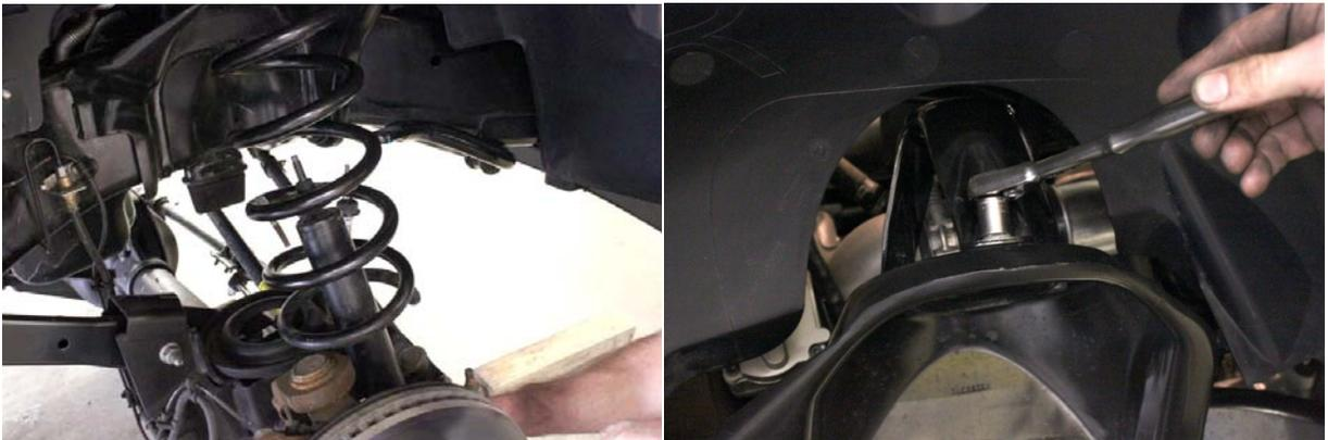
6. Install Coil Spring Spacer into upper spring mount with upper shock mount in original position, tight to factory specs with new hardware provided. Reinstall Rubber spring isolator.
