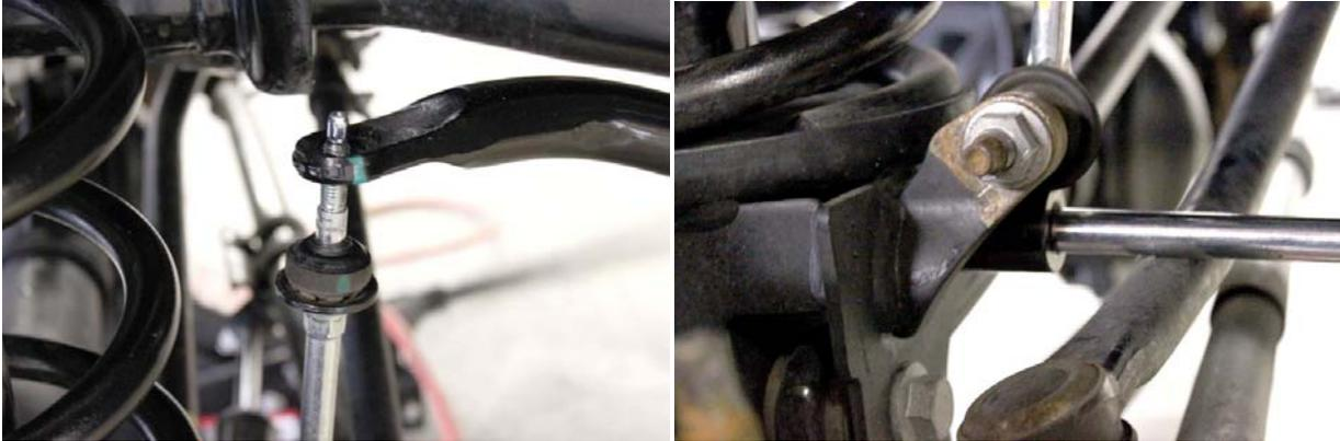
4. Lower the axle to remove the shock from the mount, then loosen the top shock mounts nuts so the shock can be removed. Lower the axle enough to remove the spring.
