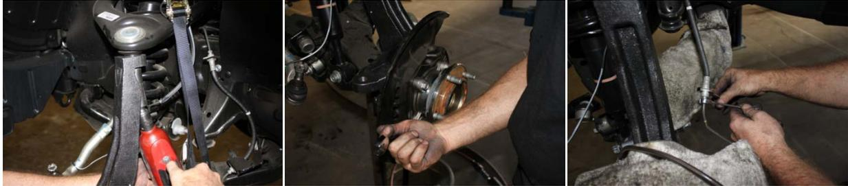
13. Reinstall brake line bracket to new spindle, you may need to bend the factory brake clip for more tension during the re-install. Bleed brakes thoroughly once everything is installed.
