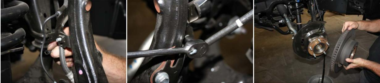
4. Unbolt wheel bearing and remove along with the dust shield.
