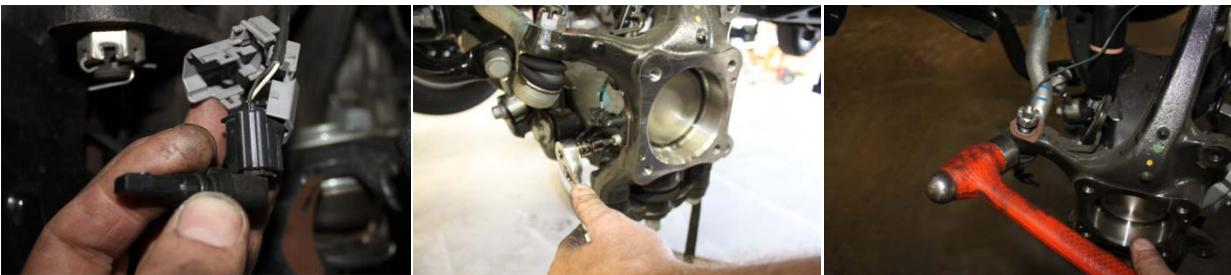
7. Loosen upper ball joint nut, but do not remove completely. Break upper ball joint loose by hitting the side of the spindle with a hammer. Once loose, remove the nut from the ball joint, and separate from the spindle.
