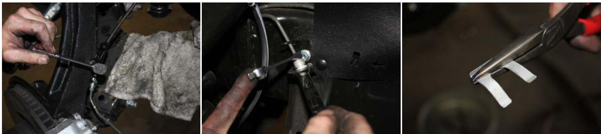
14. Install ABS sensor using the factory bolt. Then guide the ABS wire up the side of the spindle using the provided clamps and hardware. Be sure to leave slack from the control arm to the spindle and cycle the spindle back and forth to insure the wire doesn't get pinched or stretched.
