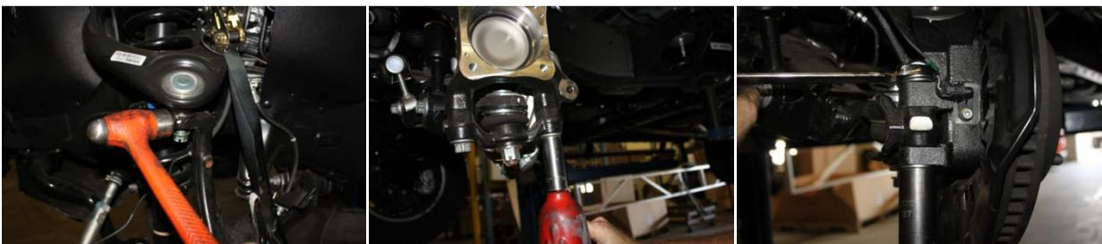
10. Attach upper ball joint using original hardware, tighten, and re-insert factor cotter pin.
